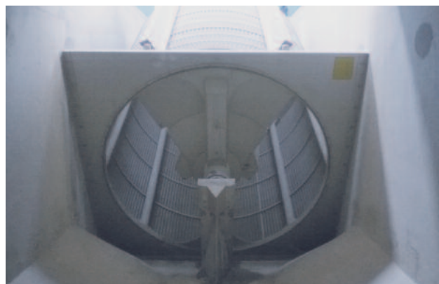
The RPPS Star liquid design with folded screen basket surface provides up to 30% higher throughput capacities with perforations of 1 / 1.5 / 2 mm.
