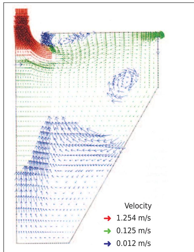
*Flow velocities in the HUBER Coanda Grit Washer RoSF4 (measured by TU Munich)*
