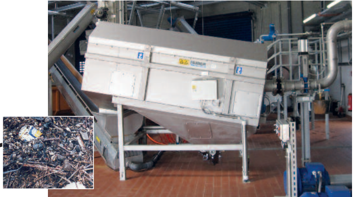
HUBER Wash Drum RoSF9 for washout and separation of all coarse material > 10 mm
