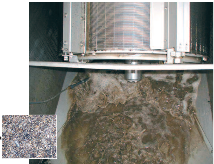
HUBER Rotary Drum Fine Screen ROTAMAT® for 1 mm screening and dewatering of organic material (approx. 30 % DR)
