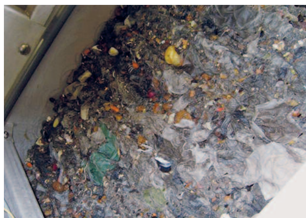
HUBER Fine Screen STEP SCREEN® SSF: high separation efficiency due to the narrow slot width and the produced screenings carpet, self-cleaning effect due to a moveable lamella unit.
