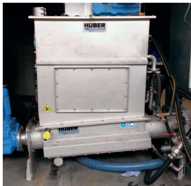
HUBER Wash Press WAP® liquid with replaceable perforated plate insert with apertures of 0.75 / 1 / 1.5 mm
