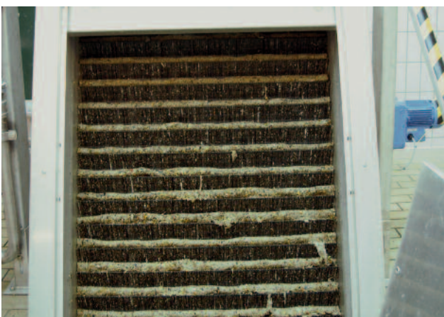
HUBER Fine Screen STEP SCREEN® SSV: very high separation capacity due to the fine slot widths and the produced screenings carpet.
