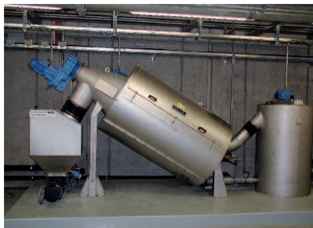
ROTAMAT® Screw Thickener RoS 2 – exceptionally robust thickener
