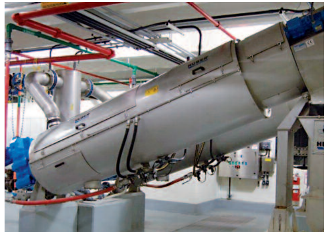
ROTAMAT® Screw Press RoS 3 Specific power consumption < 10 kWh/t DR
