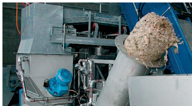
Well washed and virtually odorless screenings from a HUBER Screenings Wash Press WAP/SL, compacted to 50 % DS
