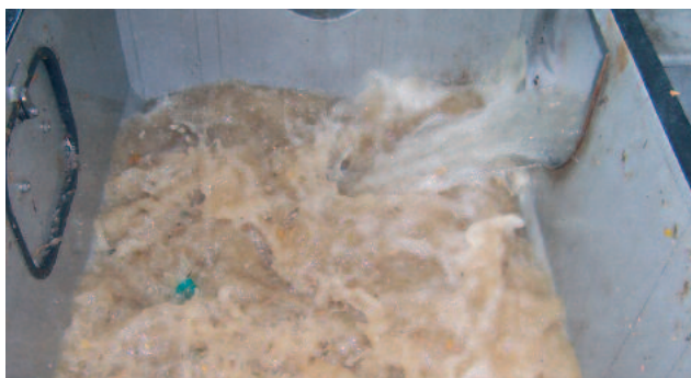
High turbulence in the launder tank during impeller operation
